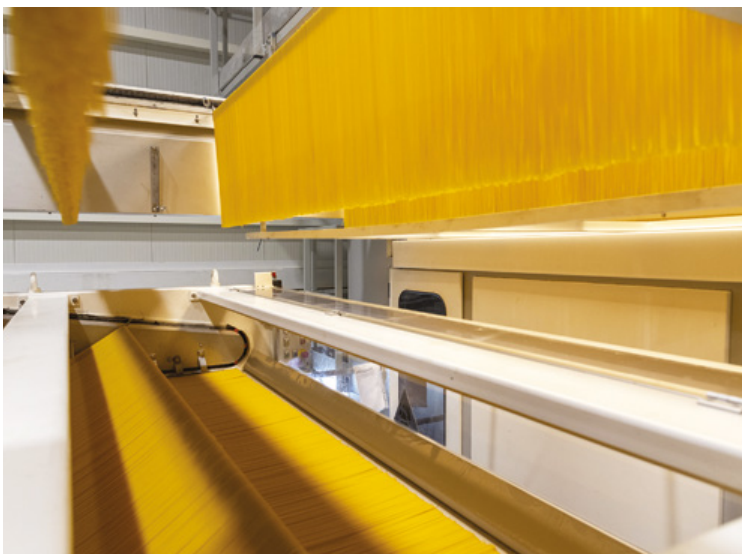
Sticks from silo to double stripper (Fava).
