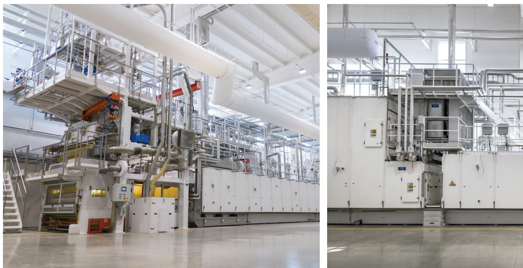
4000 kg/h long-cut pasta line GPL 180 and a detail of cooling inlet zone (Fava Storci).
