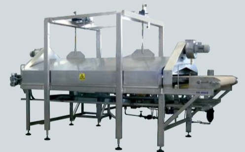
THERMAL TREATMENT LINE FOR REGIONAL PASTA SHAPES (ORECCHIETTE)
