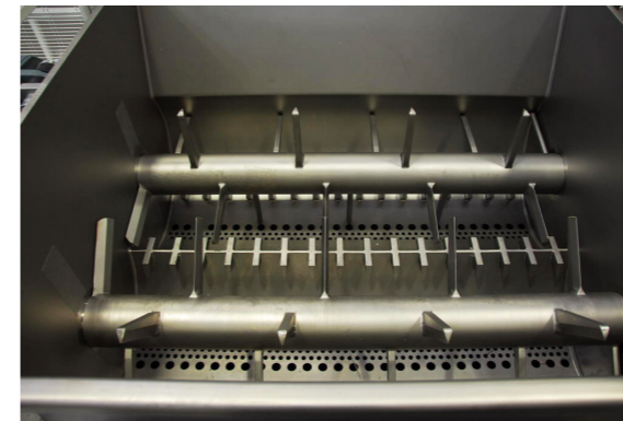
Shaft of the tank
