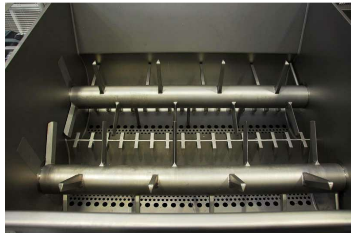
Shaft of the tank
