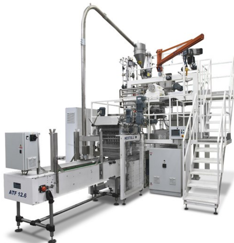
■ Trays feeder for nests/lasagna line
