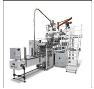
Trays feeder for nests/lasagna line
