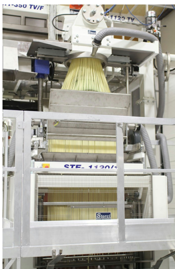
Application of spreading machine STE 1120 on Omnia line with "mushroom head" spreader
